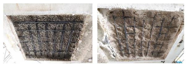
Fig. 7 Spalling of RC Slab for RWS : Reference(L) and Fire-proofed(R)
