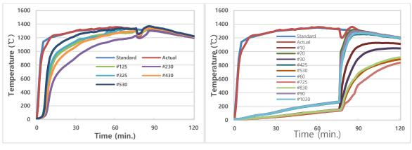
Fig. 5 Time-Temperature Curves for RWS : Reference (L) and Fire-proofed (R)
