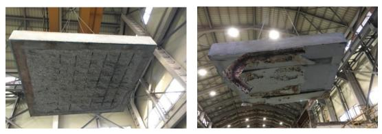
Fig. 6 Spalling of RC Slab for RWS : Reference(L) and Fire-proofed(R)
