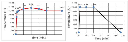
% Two curves have been used to imitate tanker fire in Netherland and Germany, respectively. Fig. 2 RWS (L) and RABT (M) Fire Load Curves
